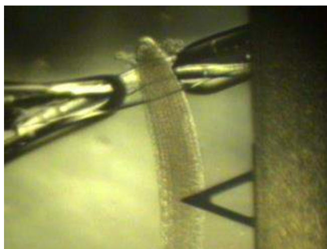
Figure 1. Root tip of an Arabidopsis thaliana seedling fixed on a glass slide using a silicon-based pressure-sensitive adhesive. The triangular shape of a PNP cantilever is located near the root transition zone, approximately 500 \mu\text{m} away from the root tip. Nanoindentation is performed on living seedlings, which presents a series of challenges as previously outlined [5].
