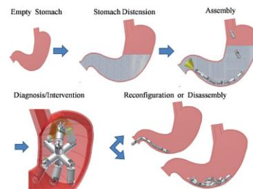
Fig. 2. Concept of the internal reconfigurable robot.
