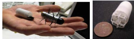
Fig. 1. (Left) Legged capsule for crawling through the colon; batteries are included in the tender module. (Right) Swimming wireless capsule for stomach exploration.
