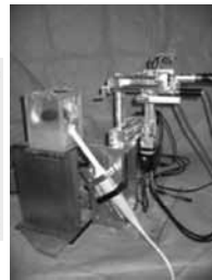
Prosper: a robot for prostate brachytherapy
